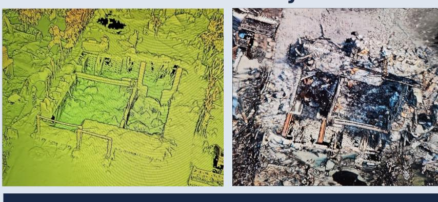
Using UAS and LiDAR to identify basement structures post-wildfire
