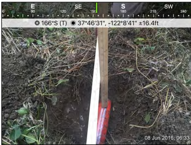
Photo 1 – QC Seed #1 placement, ~8” bgs orientated parallel to the transect.
