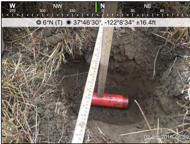
Photo 1 – QC Seed #2, med ISO (sch40 2"x8") placement, ~10" bgs orientated perpendicular to the transect.
