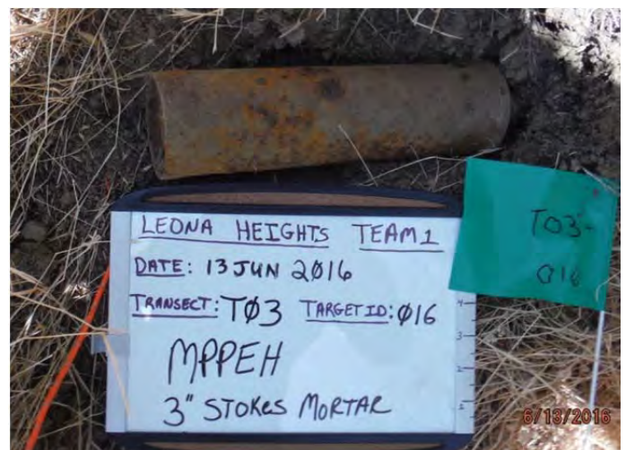
Photo 12 – T03-016 MPPEH 3" Stokes Mortar, ~2" bgs.
