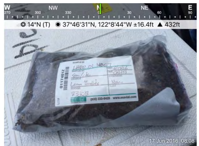
Photo 6 – Pre-demolition soil sample successfully collected, labelled, and packaged for transportation to lab.
