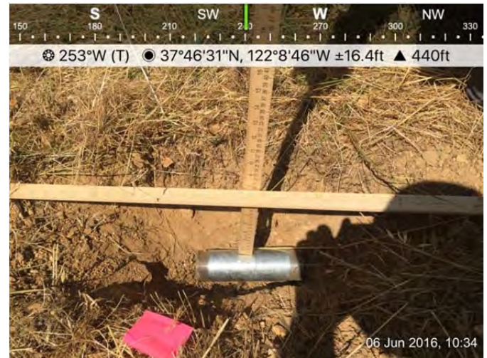
Photo 4 – ITS seed #2 (Medium ISO, 2"x8" schedule 40) ~8" below ground surface (bgs) orientated perpendicular to travel path.
