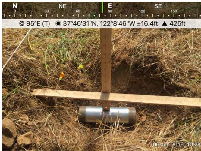
Photo 3 – ITS seed #1 (Medium ISO, 2"x8" schedule 40) ~4" below ground surface (bgs) orientated perpendicular to travel path.
