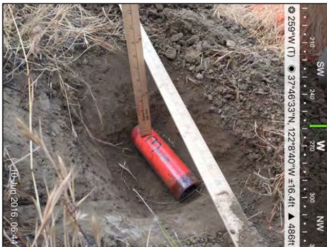
Photo 1 – QC Seed #3, med ISO (sch40 2"x8") placement, ~8" bgs orientated perpendicular to the transect.
