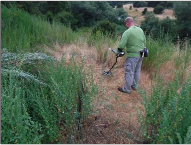
Photo 1 – UXO tech testing White's all metal detector across the instrument test strip (ITS).
