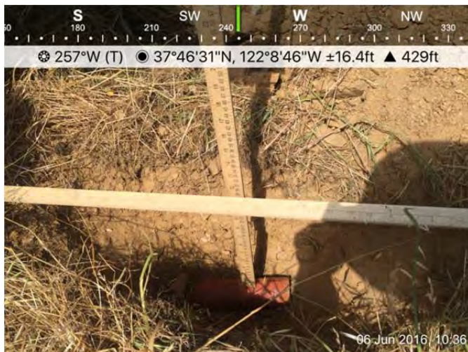
Photo 5 – ITS seed #3 (Medium ISO, 2"x8" schedule 40) ~12" below ground surface (bgs) orientated perpendicular to travel path.
