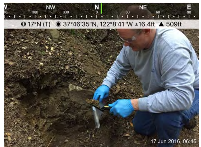
Photo 4 – Collecting pre-demolition soil sample from demolition area.
