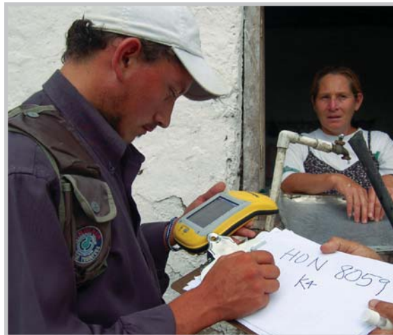
The automated data system included GPS receivers, Tablet PCs, and the ability to upload data nightly to the AuditFast Web site to compile precise information about each water system.
