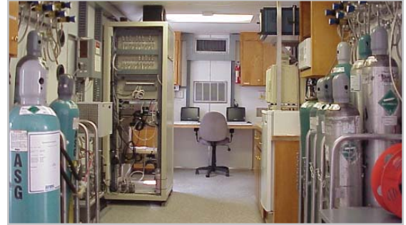
The mobile CEMS laboratory is equipped with an integrated calibration gas flow control system.
