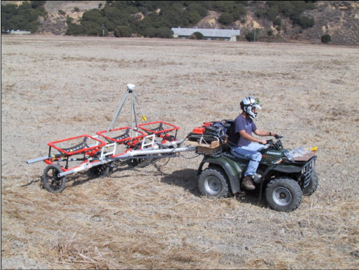
Figure 1: Multi-unit array (three sensors) of EM61-MK2 metal detectors pulled with an ATV.
