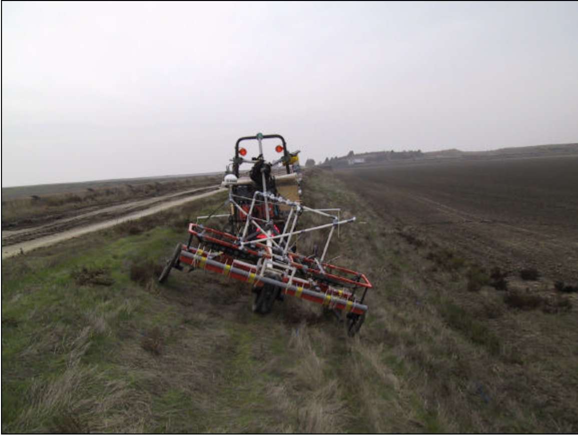
Figure 2: Dual unit array (two sensors) of EM61-MK2 metal detectors pulled with an articulating mower along berm slope.
